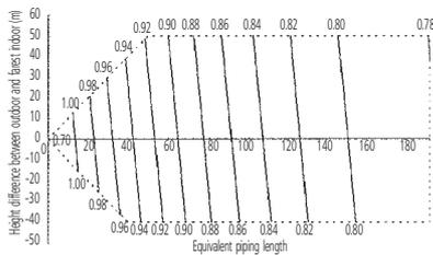
• Correction ratio for heating capacity
