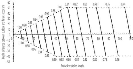
• Correction ratio for heating capacity
