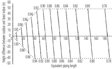
• Correction ratio for heating capacity
