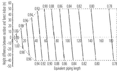
• Correction ratio for heating capacity
