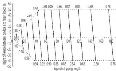
• Correction ratio for heating capacity
