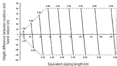
Correction ratio for heating capacity
