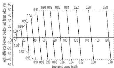
• Correction ratio for heating capacity
