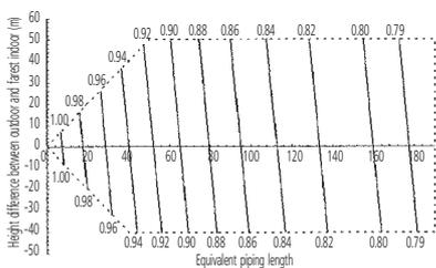
• Correction ratio for heating capacity
