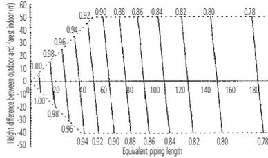
• Correction ratio for heating capacity
