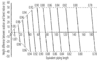
• Correction ratio for heating capacity
