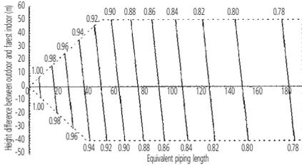
• Correction ratio for heating capacity
