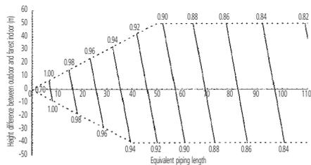
• Correction ratio for heating capacity
