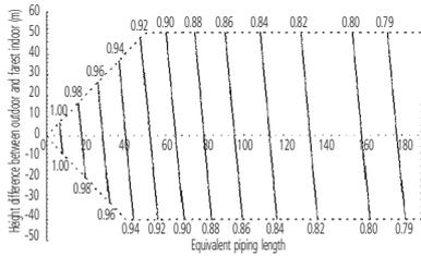
• Correction ratio for heating capacity
